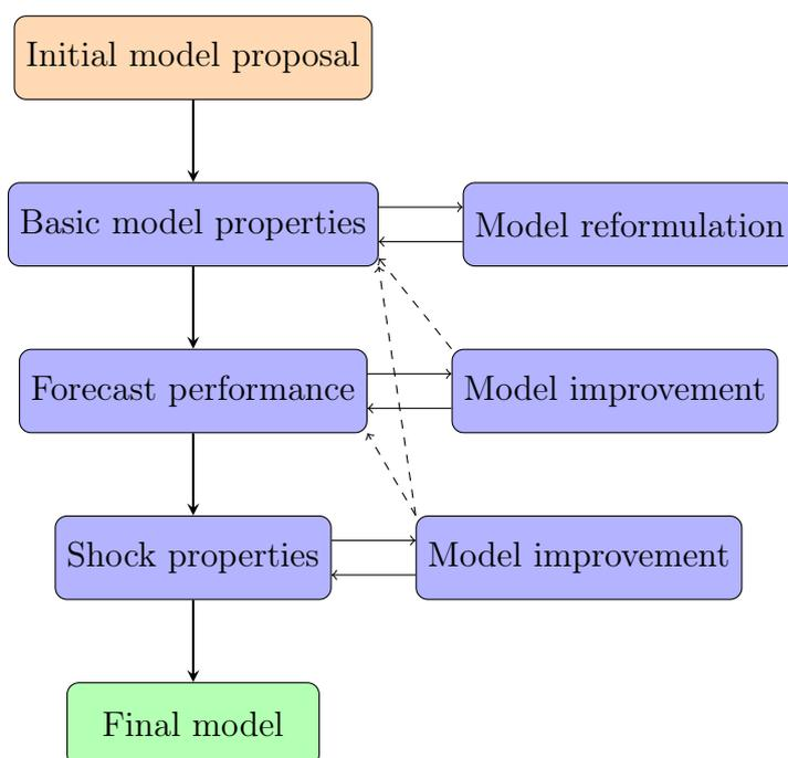
The process starts with an initial proposed model, which is then evaluated using the outputs of the add-in. The initial model is best evaluated by looking at the forecast summary graphs, which allow the model developer to visualize the model forecasts and compare them with the actual values, and hence obtain some qualitative notion of forecast quality and errors: when only a single model is being
